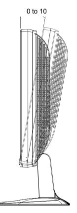
Figure 1-3: Tilting the Monitor
